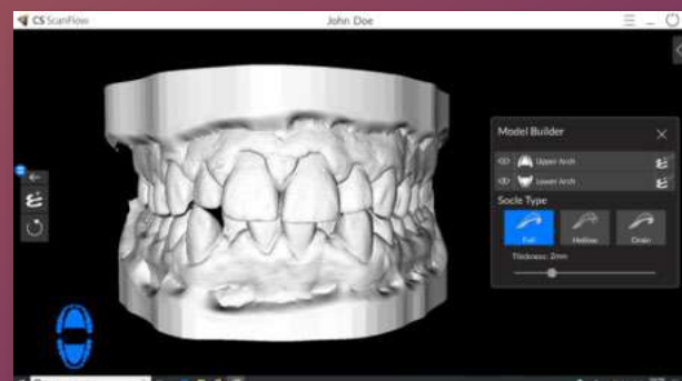
Add a base to your digital impression using Model, which can be used for 3D printing.*
